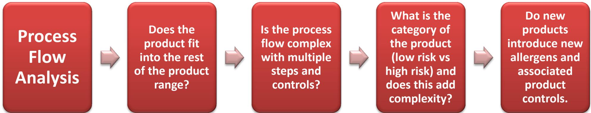
**Process Flow Analysis** is used to help fully understand the current or proposed condition of any manufacturing process facility. Process Flows can be used to identify all elements within a manufacturing facility from raw materials through to people and waste routes.
